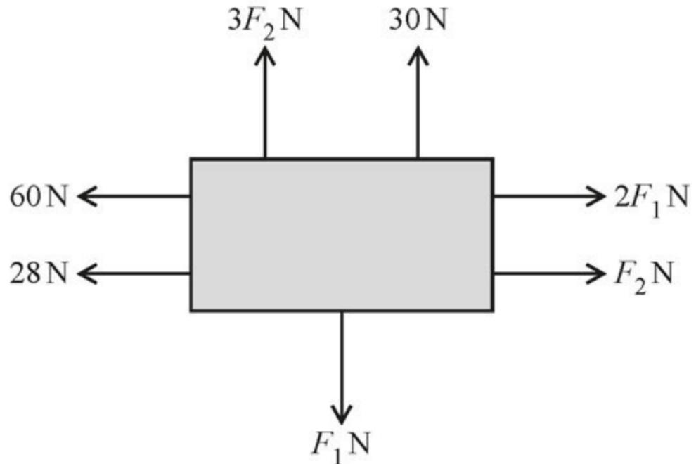
A body remains at rest when subjected to the horizontal and vertical forces shown in the diagram.
