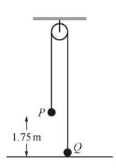
Particles P and Q, of masses 4 kg and 6 kg respectively, are attached to the ends of a light inextensible string. The string passes over a smooth fixed pulley. The system is in equilibrium with P hanging 1.75 m above a horizontal plane and Q resting on the plane. Both parts of the string below the pulley are vertical (see diagram).
