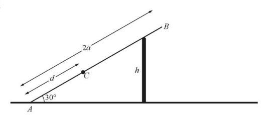
The diagram shows a ladder AB, of length 2a and mass m, resting in equilibrium on a vertical wall of height h. The ladder is inclined at an angle of  $30^{\circ}$  to the horizontal. The end A is in contact with horizontal ground. An object of mass 2m is placed on the ladder at a point C where AC = d.
