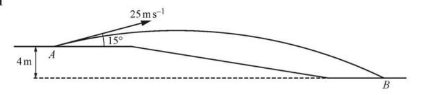
A golfer hits a ball from a point A with a speed of  $25 \,\mathrm{m \, s^{-1}}$  at an angle of  $15^\circ$  above the horizontal. While the ball is in the air, it is modelled as a particle moving under the influence of gravity. Take the acceleration due to gravity to be  $10 \,\mathrm{m \, s^{-2}}$ .
