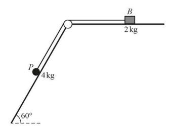
The diagram shows a small block B, of mass  $2 \, \text{kg}$ , and a particle P, of mass  $4 \, \text{kg}$ , which are attached to the ends of a light inextensible string. The string is taut and passes over a small smooth pulley fixed at the intersection of a horizontal surface and an inclined plane. The particle can move on the inclined plane, which is rough, and which makes an angle of  $60^{\circ}$  with the horizontal. The block can move on the horizontal surface, which is also rough.
