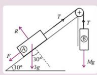
For A: Resolving perpendicular ( $^{\nwarrow}$ ):  $F_{\text{net}} = ma$
